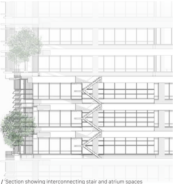
/ Section showing interconnecting stair and atrium spaces
