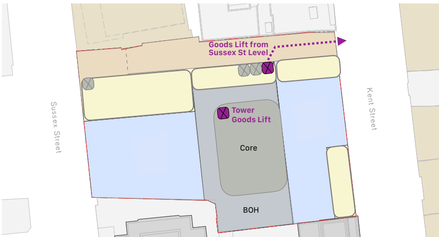
/ Plan Diagram Kent St Level - Goods Lift Connection at Kent St Through Site Link
